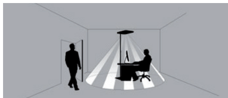
Fig. 12: Detection range of the PIR sensor.
