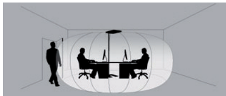
Fig. 11: Detection range of the HFMD.
